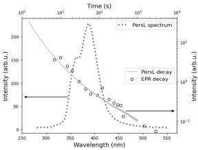
PersL spectrum of  $Sr_3MgSi_2O_8$ : Ce<sup>3+</sup> and comparison of paramagnetic center signal time-derivative decay with PersL kinetics.
